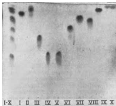
Fig. 1.—Chromatoplate of penicillins (I-X) in system A.
